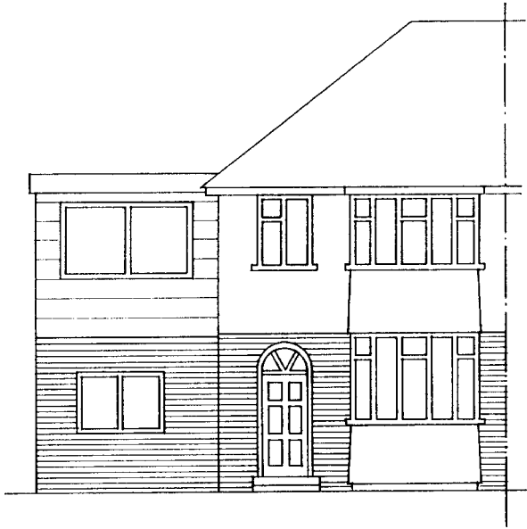
Extension is not integrated
