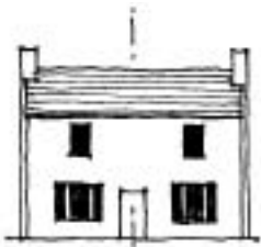
Before .... A symmetrical facade of vertically proportioned windows
