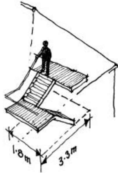
A staircase takes up a large volume: in a bungalow this may mean the loss of valuable floorspace
